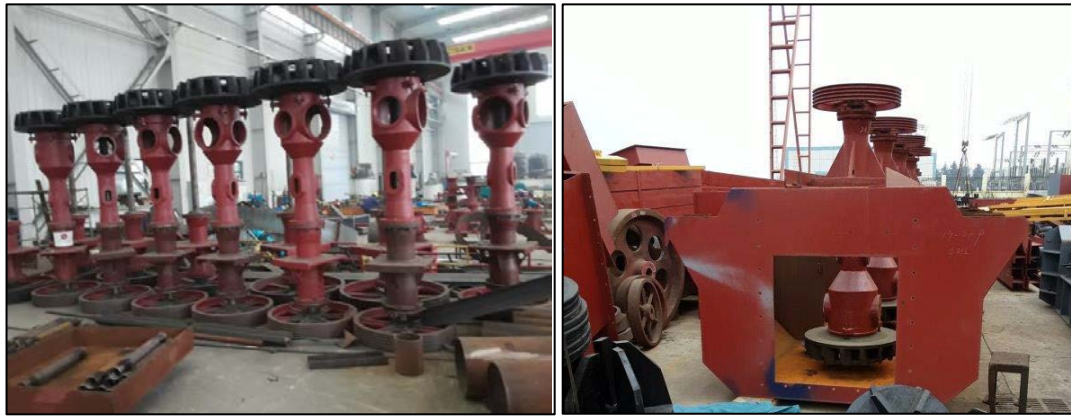
Figure 4: Equipment manufactured at Jinpeng Engineering in Yantai, China. Flotation cell impellers in undercover storage (left) and pre-assembled flotation cell to facilitate the location and installation of the impeller guides prior to rubber lining and final assembly (right).
