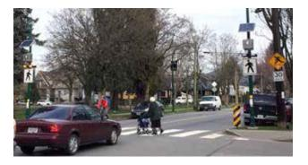
Photo: Rectangular Rapid Flashing Beacon (RRFB) at Victoria Drive and Grant Street
