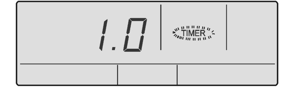
3. 3 seconds after the last press of the for buttons or simply press **TIMER**, the display will go back to the main screen and the OFF Timer countdown will start. The unit will turn Off after the timer has expired.
