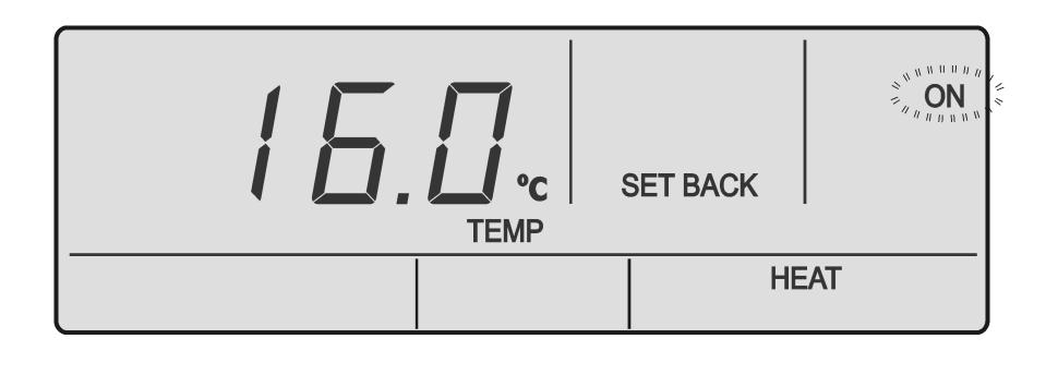
7. Press the or button to change the **HEAT** set back temperature.
