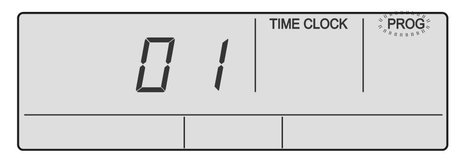
Press the PROG button to enter the time clock menu. Time clock program is currently On.
