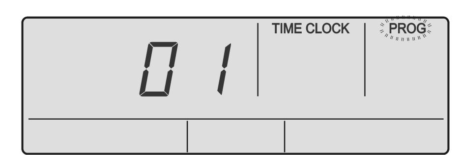
Press the **PROG** button to enter the time clock menu. **TIME CLOCK** and **PROG** indicators are still illuminated. **ON** indicator will be flashing in the screen.
