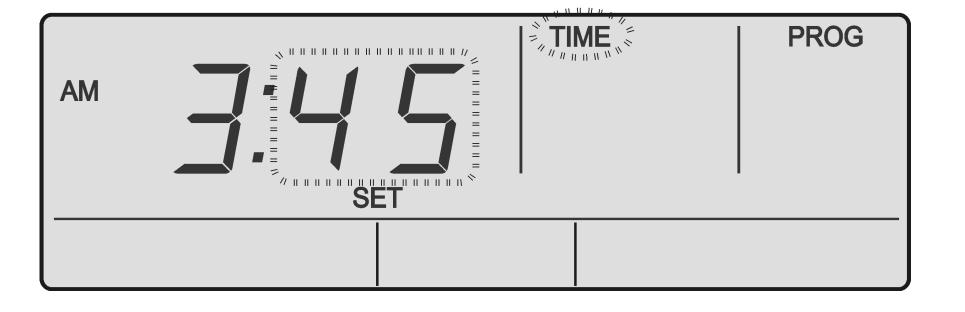
7. Press the **PROG** Button to accept the desired minutes. Day field will start blinking. Day indicator will be flashing, i.e. **MON**.
