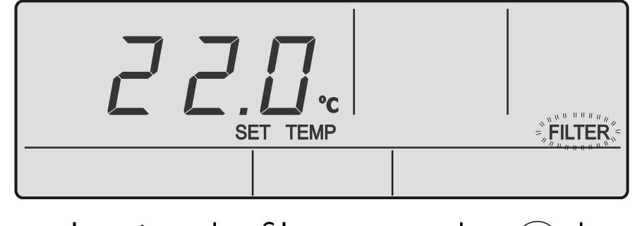
2. After cleaning the filter, press the button to reset the timer. Flashing **FILTER** display will disappear.
