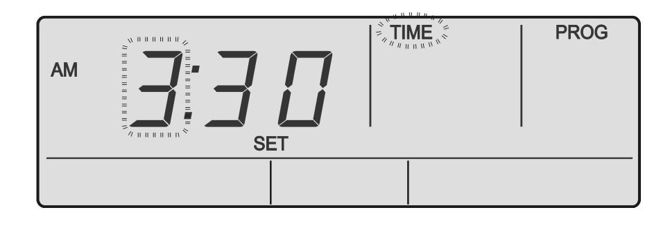
5. Press the **PROG** button to accept the desired hour. Minute field will start blinking.
