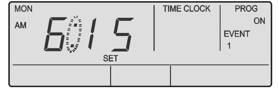
4. Press the **PROG** button to move to Event 1 Off time. Press the or button to adjust the time in 15 minutes increments.
