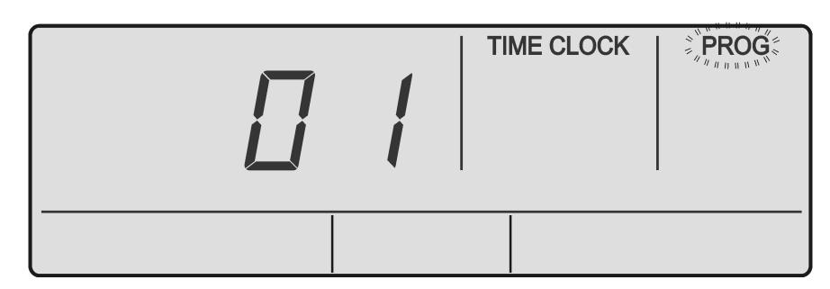
Press the PROG button to enter the time clock menu. Time clock program is currently ON.
