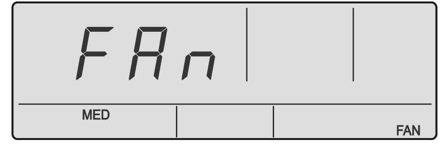
Adjust the Indoor Fan speed (LOW, MED and **HIGH**) by pressing the button successively until you reach the desired speed.
