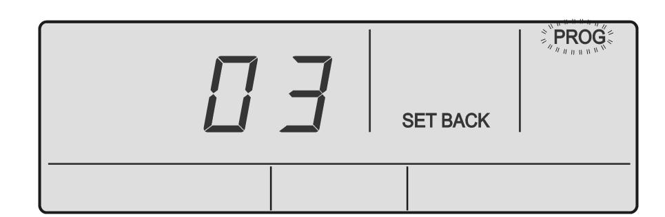
3. Press the **PROG** button to enter Program Menu O3. Display will show **SET BACK** indicator and **OFF** field is blinking.
