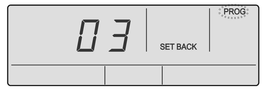
3. Press the **PROG** button to enter Program Menu O3. Display will show set back display **ON** field is blinking.
