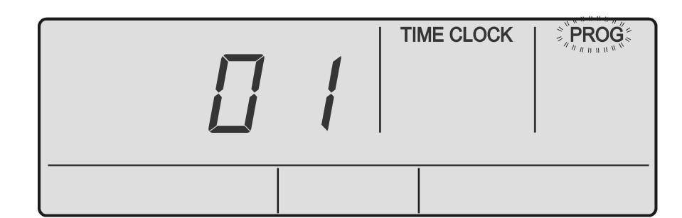
Press the PROG button to enter the time clock menu. By default, Time clock program is Off.
