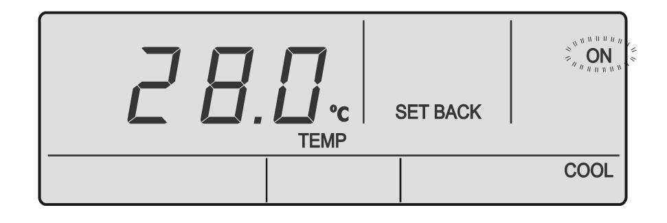
6. Press the **PROG** button to accept **COOL** set back temperature. Next screen will show **HEAT** set back temperature adjustment.
