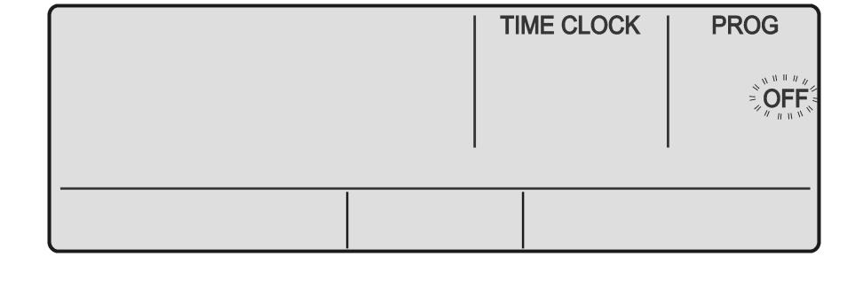
4. Press the **PROG** button to accept the selection and de-activate time clock, then press the **EXIT** button once. **TIME CLOCK** indicators will disappear from main screen, indicating that the Time clock has been de-activated.
