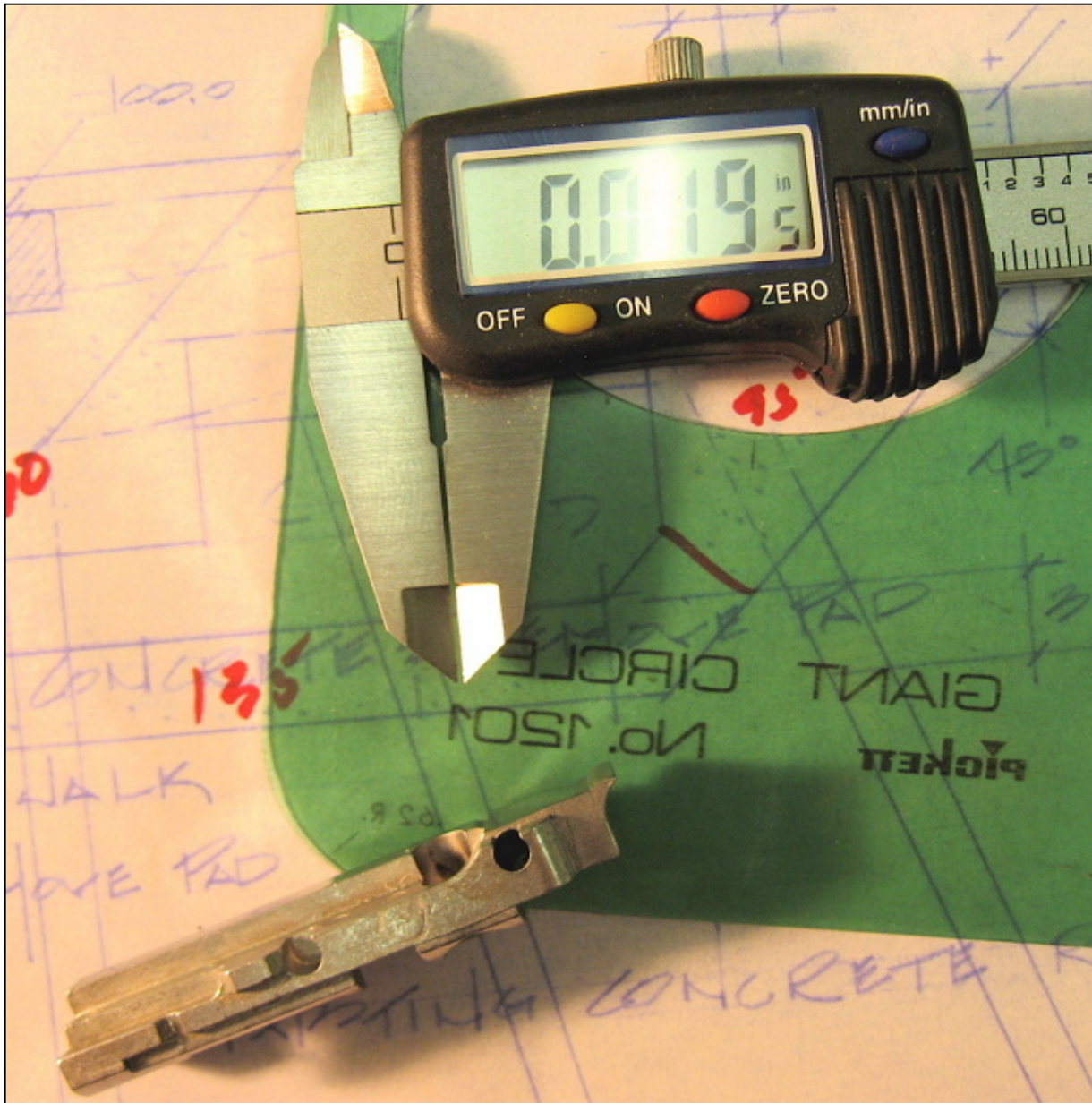
This photo shows the 0.020" of material removed from the bottom rear of the breech block.
