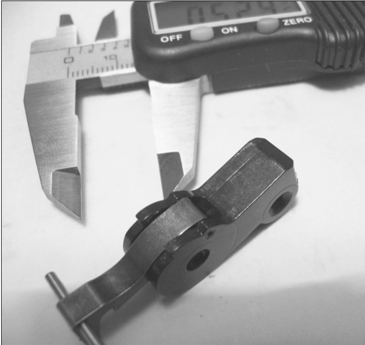
New style hammer ready for re-profiling.
