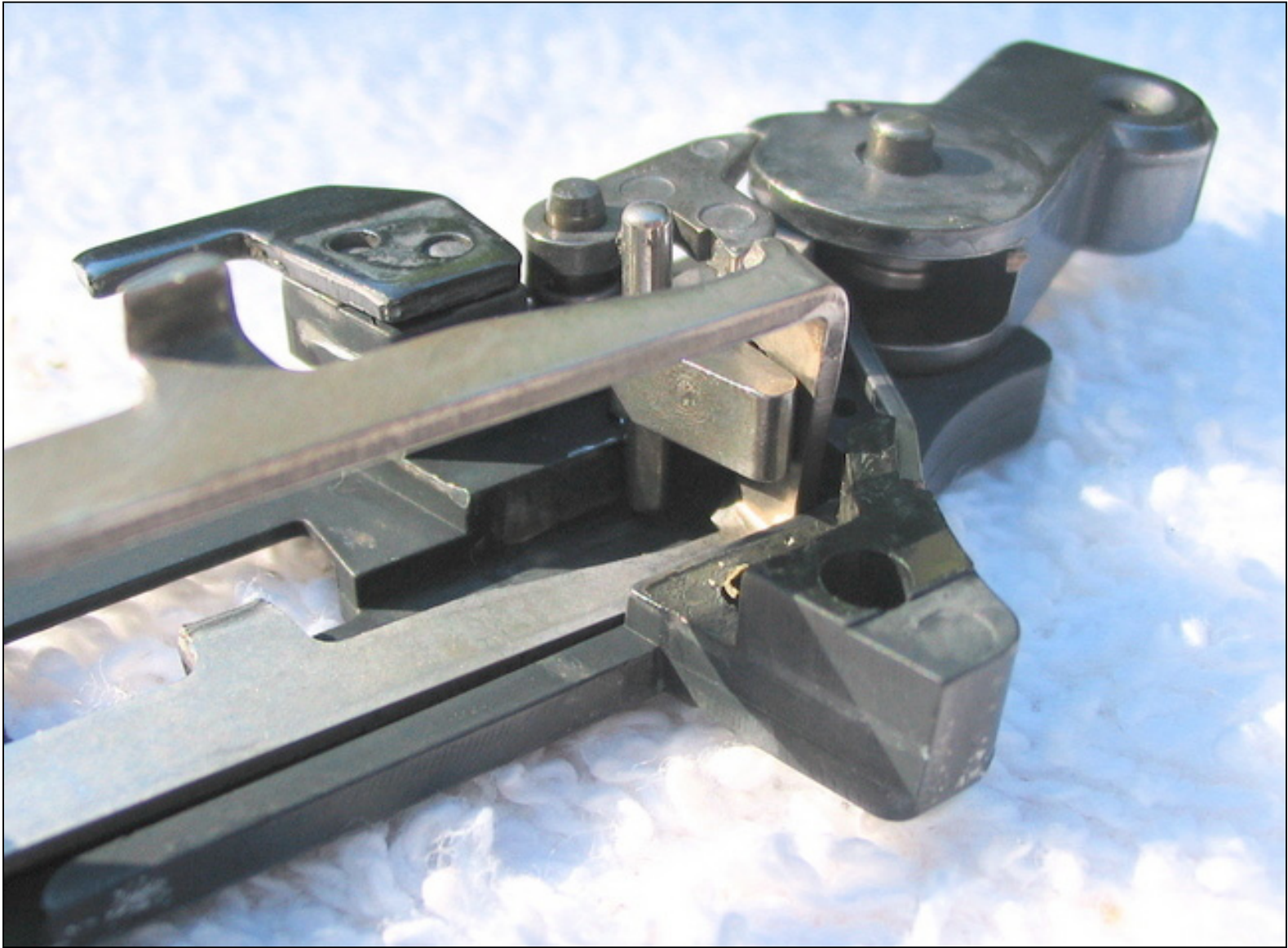
Relationship of components, assembled. Notice the fit of the hammer pin as it sits through the hammer. It must fit like this upon reassembly.
