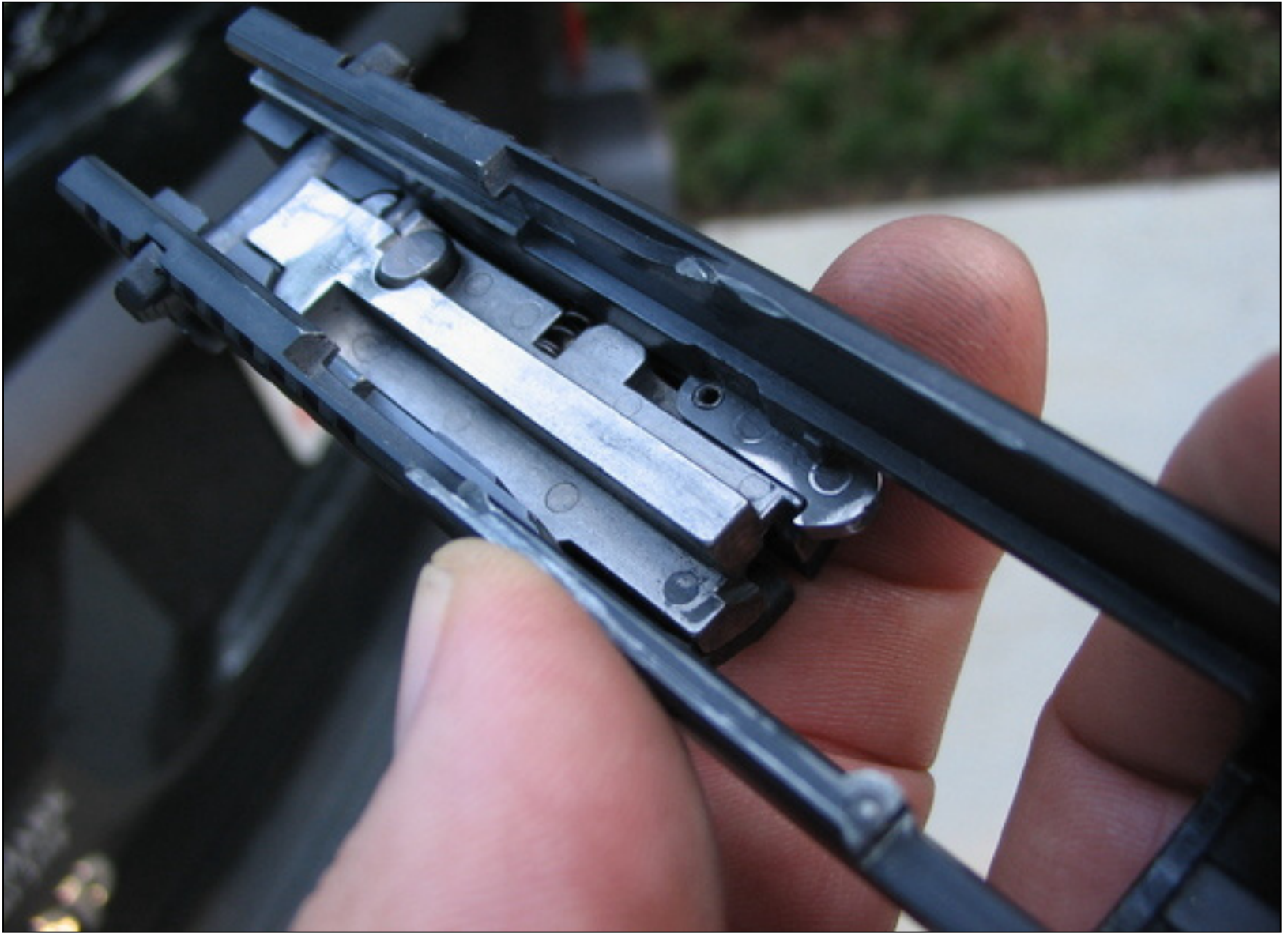
Extractor pin reinstalled and seated flush.
