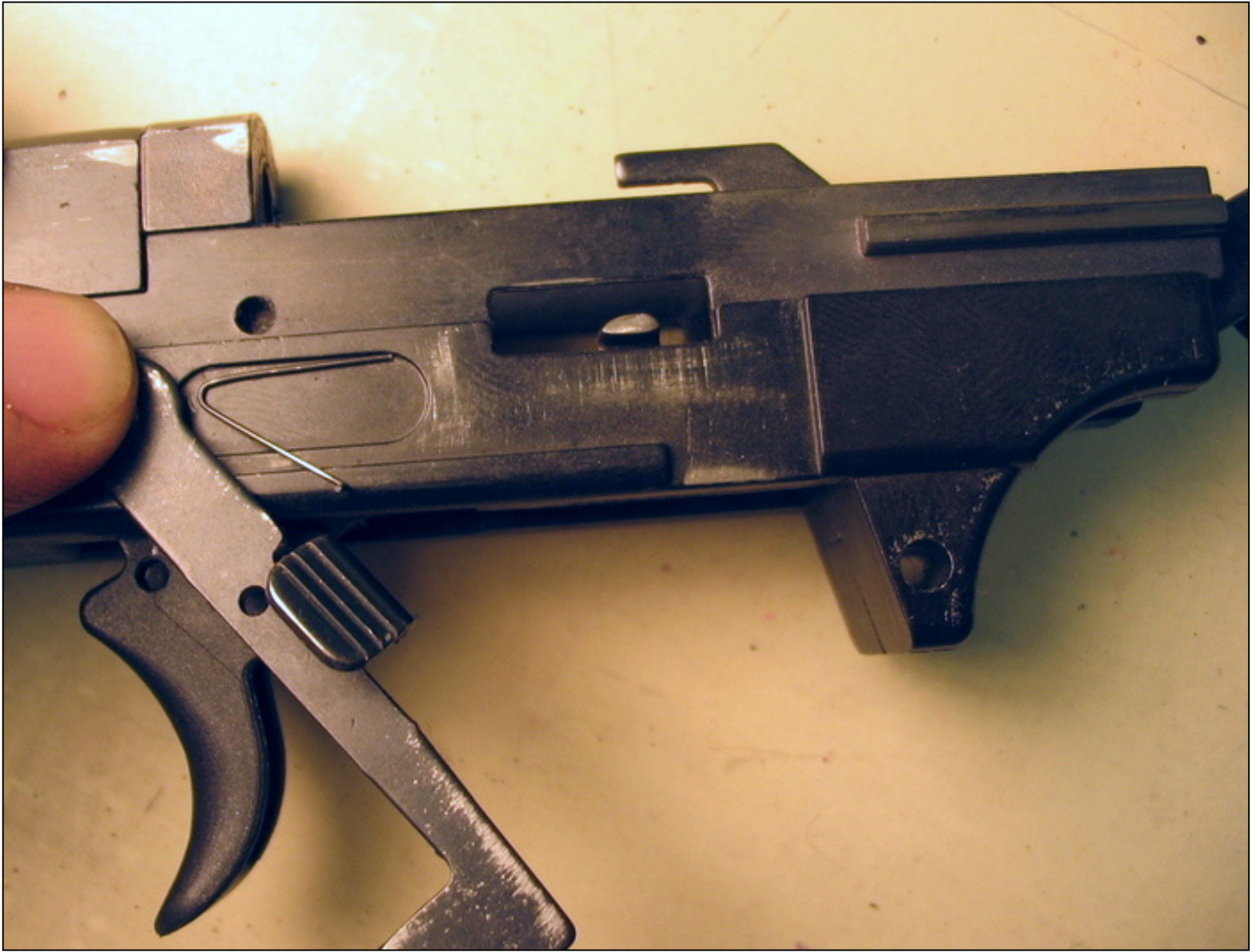
Photo of the proper position of components upon reassembly of the slide stop mechanism.
