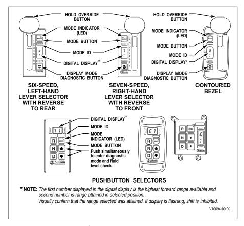
Figure 10. Allison 4<sup>th</sup> Generation Controls Shift Selectors and Pushbutton Selectors
