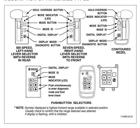
Figure 5. WTEC III Shift Selectors
