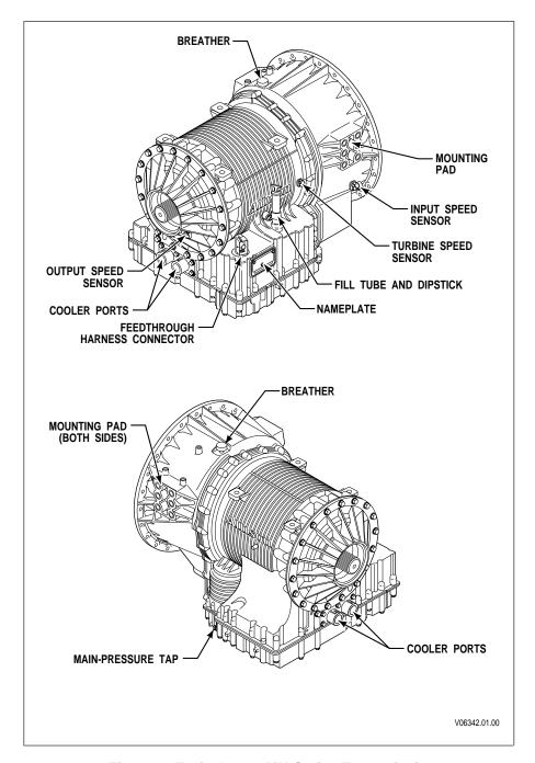
Figure 4. Typical 4000 MH Series Transmission (Allison 4<sup>th</sup> Generation Controls)
