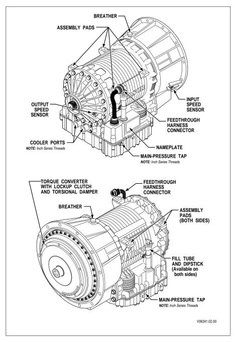
Figure 1. Typical 3000 MH Series Transmission (WTEC III Controls)
