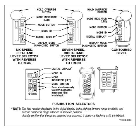
Figure 6. Allison 4th Generation Controls Shift Selectors
