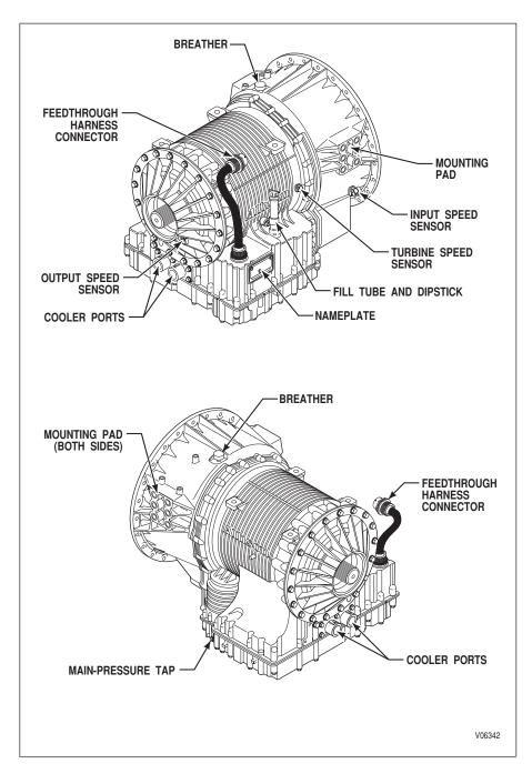
Figure 3. Typical 4000 MH Series Transmission (WTEC III Controls)
