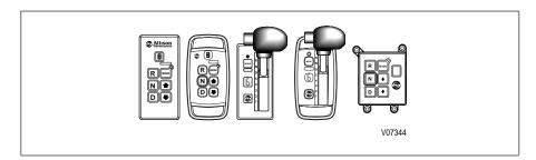
Figure 7. Typical Shift Selectors (WTEC III Controls)
