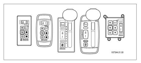
Figure 8. Typical Shift Selectors (Allison 4<sup>th</sup> Generation Controls)
