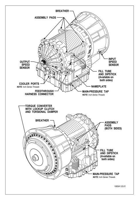
Figure 2. Typical 3000 MH Series Transmission (Allison 4<sup>th</sup> Generation Controls)
