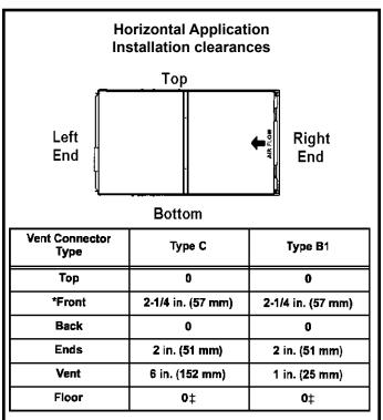
\* Front clearance in alcove installation must be 24 in. (610 mm). Maintain a minimum of 21 in. (610 mm) for front service access. ‡ For installations on a combustible floor, do not install the furnace directly on carpeting, tile or other combustible materials other than wood flooring.
