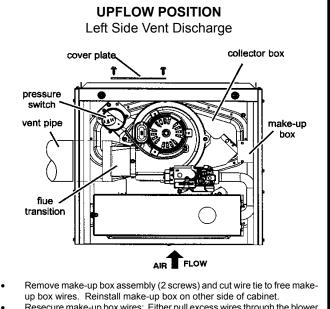
Resecure make-up box wires: Either pull excess wires through the blower compartment and secure using supplied wire tie, or coil excess wire and secure to the gas manifold.
