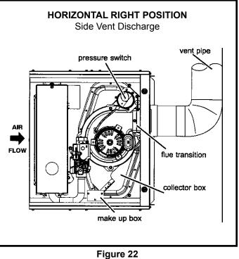
These series units are classified as fan assisted Category I furnaces when vertically vented according to the latest edition of National Fuel Gas Code (NFPA 54 / ANSI Z223.1) in the USA. A fan assisted Category I furnace is an appliance equipped with an integral mechanical means to either draw or force combustion products through the combustion chamber and/or heat exchanger. This unit is not approved for use with horizontal venting.
