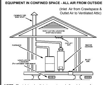
**NOTE:** The inlet and outlet air openings shall each have a free area of at least one square inch per 4,000 Btu (645 mm<sup>2</sup> per 1.17 kW) per hour of the total input rating of all equipment in the enclosure.
