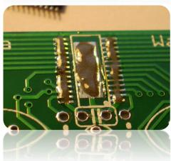
3. As you can see, it doesn't look pretty and it doesn't have to! You can also put some solder paste on the pin's locations so you don't have to use a soldering iron after "hot-plating" the IC. You will see what "hot-plating" is later on.
