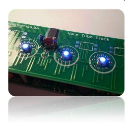
1. Make sure your desk is clean of all wires and solder remains, and plug in the DC supply to the "main board" and the LEDs should start blinking in blue after few seconds!
