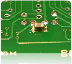
2. While holding it down on the PCB, solder just one side.
