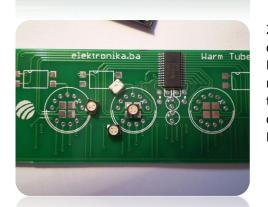
2. Place the LED in the position but keep in mind about its common Anode pin. The common Anode is marked on the PCB as you can see – the upper right corner has a white mark. The first pin on this RGB LED is actually a Cathode of the RED LED-part, so by following the IC marking convention the common Anode is the fourth pin of this RGB LED.
