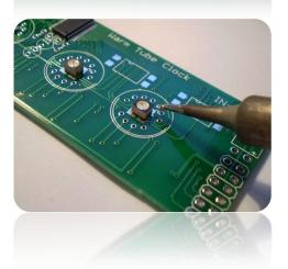
3. After placing the LED in its position, you can hold it in place using tweezers while firstly soldering it's any pin ("tacking" it actually). After "tacking" it into place with some solder, you can solder the remaining pins and then go back to solder the "tacked" pin. While soldering these LEDs, you actually don't need to touch the LED with the soldering iron. It is enough to touch the PCB under the LED's pin and it will solder it.
