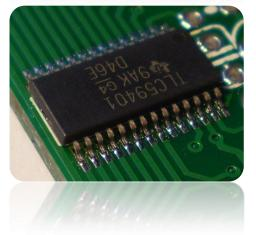
10. Now it is time to remove the PCB from the "hot-plate". I usually don't leave it there until it cools down totally, so after turning the "hot-plate" off I wait about half a minute and remove the PCB with hands, but very slowly, and place it on the desk to cool down.
