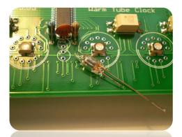
1. This is a Nixie dot. It is actually a neon lamp that lights up when you supply it with more than 100V DC. We will be lighting it up with around 185V so that's why we used those 910k resistors. You can actually increase the value of those resistors to lower the current through these neon lamps even more.
