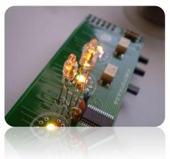
4. Now solder the "upper dot" behind it. It should go around **21.3mm** from the top of the PCB.
