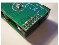
2. Push it all the way down while soldering, so it doesn't "float"! Simply solder both connectors while the PCB is on top of the "main board" like in the picture.
