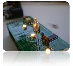
3. After soldering one dot, you probably can't wait to try it out! So, plug in the DC power supply and check it out! It should blink in ½ Hz interval.
