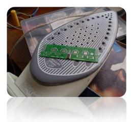
8. Place the PCB onto the "hot-plate" and turn it ON to pre-heat. Don't turn the "hop-plate" to maximum temperature just yet. First put it to half, wait a minute, and then turn it up to the maximum. The maximum temperature for a clothing iron is around 210 degrees Celsius which is just enough to get the job done.
