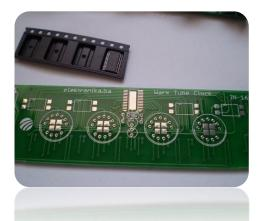
1. Make sure the PCB pad where IC goes is clean from grease. Rub it with some alcohol just in case.
