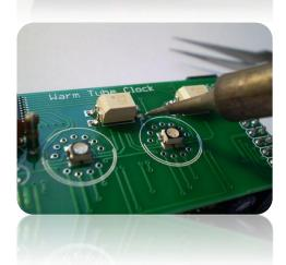
2. Place them correctly and in proper orientation and while holding with tweezers, solder ("tack") just one pin of each opto-coupler to hold them in place.
