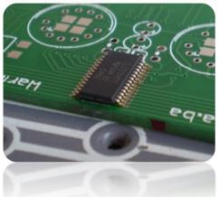
9. Now, what you can (should be able to) see in this picture is that the soldering paste we previously applied is slightly starting to melt and liquefy. It might also start to smoke a bit (depends on the type of your liquid solder) – so don't worry that is normal.
