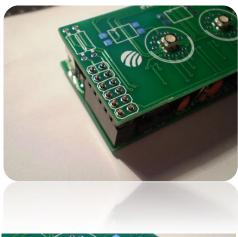
1. Put these into the female pin headers on the "main board", all the way in. Now place the shield board on top of the "main board" like in the picture. This way you will know that it will fits perfectly!
