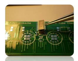
4. Now, using your tweezers gently place the component in its position. Push it all the way to the PCB so it kind of "glues" itself. Make sure it is centred and placed correctly!
