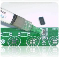
2. Apply <u>some</u> amount of liquid solder paste. I can't give you the exact amount of solder paste to use, as this comes with experience and pure sense.
