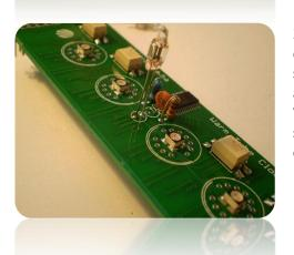
2. For the IN-16 Nixie tube, you should solder the "lower dot" at a distance of **12.65mm** from the PCB. When you solder the IN-16 Nixie tubes, you will see if you need to readjust the height of the Nixie dots.
