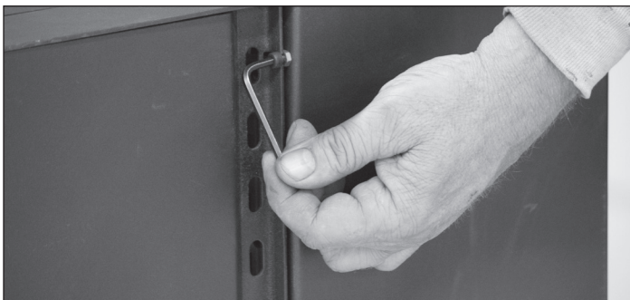
Figure 36: Remove side panel screws using 1/8 allen wrench
