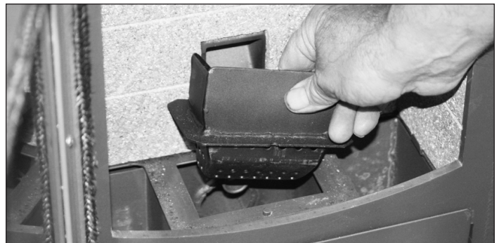
Figure 30 : Fire pot clean
