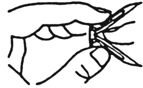
Fig. 18 - Popping Open Anchor Wing For Thin Walls
