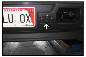
13. Optional: Prior to fully reinstalling the fascia. Drill a hole thru the bumper at the deisired location to accomodate the plug and bolts. Using 1/4" x 1-1/2" bolts with 1/4" washers, install the plug thru the bumper. On the backside of the bumper, install the electrical bracket and 1/4" locknuts to secure the plug to the bumper.
