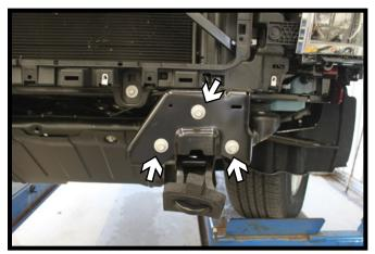
Using a 15MM socket, remove the three (3) bolts from the cover plate. Do this on both sides of the vehicle.
