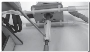
Slip the drive shaft out of the back of the boat. Wipe off any grease and water that might be on the shaft.
