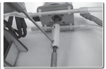
Now is also a good time to place a drop of light oil on the motor bearing.
