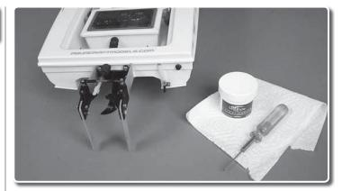
Using a 1.5mm hex wrench, loosen the set screws holding the drive cable to the motor coupler. It is important to note that there are two set screws holding the cable in position.
