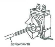
Caution: One full counterclockwise turn of the calibration screw will increase the shut off temperature approx. 7 degrees. Never turn the calibration screw more than five revolutions. This will damage the thermostat!
