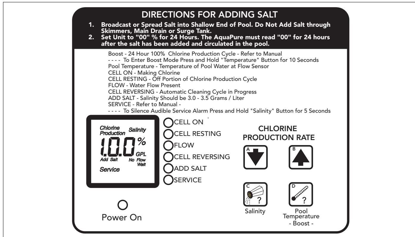
Figure 13. Control Center Front Panel
