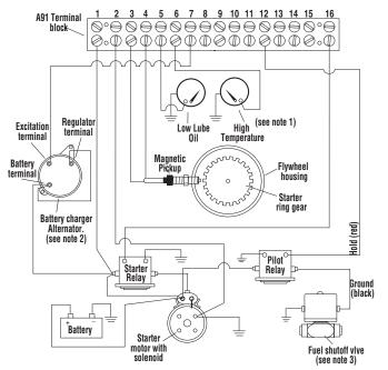
Oil pressure and water temperature SWICHGAGE® instruments are shown for simplicity. Any sensor for oil pressure, or level, or water or oil temperature can be used, as long as its contacts are open to run, and close to ground for shutdown lockout.
