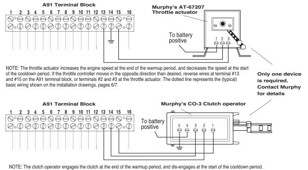
The dotted line represents the (typical) basic wiring shown on the installation drawings, pages 6/7.
