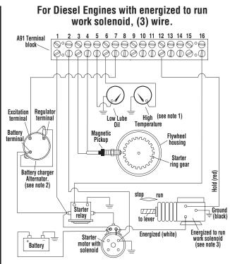
Oil pressure and water temperature SWICHGAGE<sup>®</sup> instruments are shown for simplicity. Any sensor for oil pressure, or level, or water or oil temperature can be used, as long as its contacts are open to run, and close to ground for shutdown lockout.
