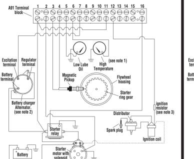
Oil pressure and water temperature SWICHGAGE® instruments are shown for simplicity. Any sensor for oil pressure, or level, or water or oil temperature can be used, as long as its contacts are open to run, and close to ground for shutdown lockout.
