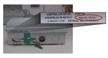
In general, Rain Bird controllers have a date code on the bottom of the external case (if they come mounted in one) and another date code on the back of the main panel.
