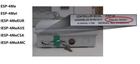
In general, Rain Bird controllers have a date code on the bottom of the external case (if they come mounted in one) and another date code on the back of the main panel.
