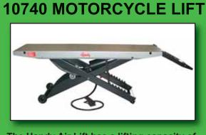
The Handy Air Lift has a lifting capacity of 1000 lbs. and an 80" x 24" deck, ideal for working on motorcycles, ATVs, snowmobiles, garden tractors, etc. It raises to a working height of 30" and lowers to 7" for easy loading. Solid steel fabrication and is powered by a pneumatic cylinder from your air source (90-100) psi. Can be used with or without accessories. W:24" x L:80". CE Approved.
