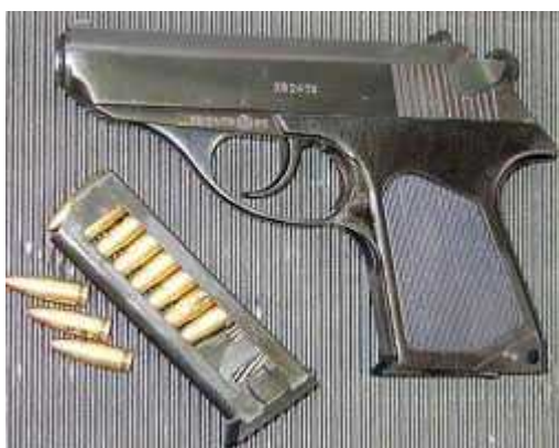
Illustration 41: PSM from the SASC Museum Collection. Note the very pointed nature of the small 5.45mmP round
