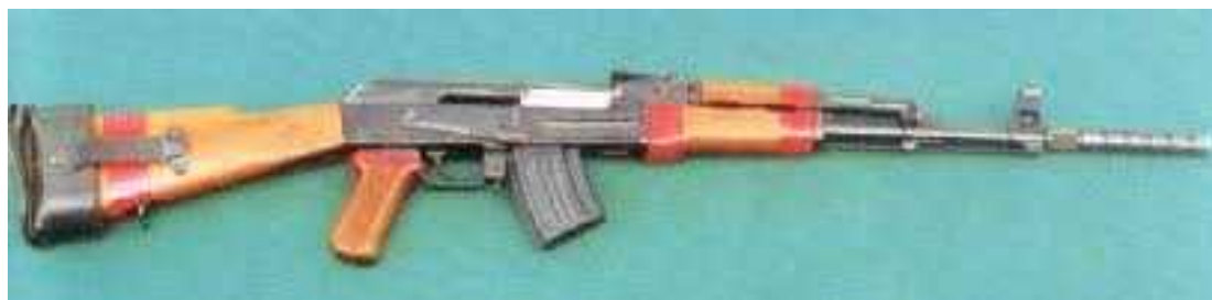
Illustration 29: Kbk Wz1960 showing butt padding and special 10 round magazine. Note the slightly different muzzle compared to the Yugoslavian version. Warsaw Collection.
