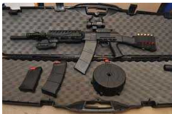
Illustration 32: Saiga12 captured and used by the US 10th SFG. It has a new hand guard to allow the fitting of a torch under the barrel, a AN/SGS2 non-magnifying sight and a but shot holder. Underneath are a 5 round magazine, a 10 round magazine and a 20 round drum. DoD
