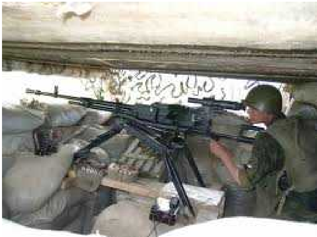
Illustration 91: NSV in a Soviet bunker on the Chinese border August 1995. Here a scope has been fitted. Note how the tripod has been weighted down. TASS
