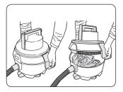
Turn off the vacuum cleaner and unplug it from the mains. Remove the hose. Unclip the retainer clips on either side of the vacuum cleaner and lift off to gain access to the dust bag compartment.
