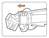
4. To start water and solution flow, push the collar on the wash tool forwards.
