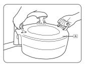
Remove clean water tank (A) from inside the dirty water tank and fill with warm (max 40°C) water to point indicated on the tank.
