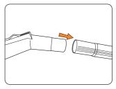
Push one end of the extension tube into the handle of the hose.
