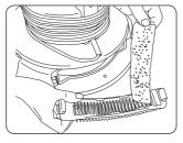
Remove the filter and wash under a tap. Allow to dry thoroughly before replacing back into the machine.
