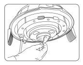
Remove the blue filter and wash under a tap. Allow to dry thoroughly before replacing back into the machine. Replace with a new filter as necessary.
