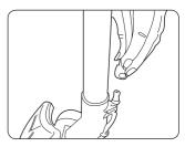
Push the second extension tube into the wash head to be used and push the end of the solution tube onto the connection port on the Wash Head / Upholstery Tool.
