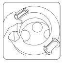
Lift out and remove the clean water solution tank. Store safely away.
