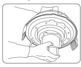
Remove the motor top from the unit, turn on its side and remove the float housing in an anti-clockwise direction to unscrew.
