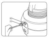
Push solution tube connector (A) firmly into solution port (A1). Twist solution tube connector (A) a quarter turn to the right to lock into place.
