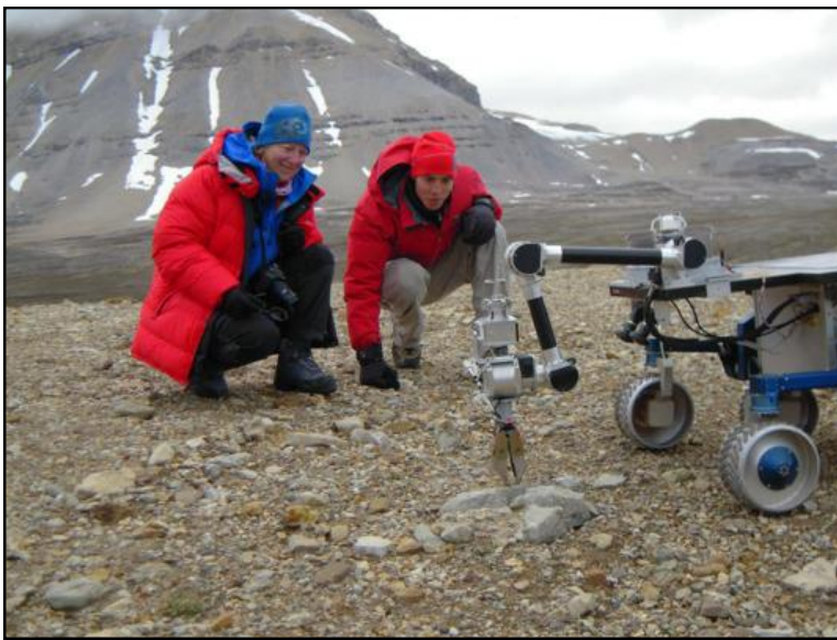
Svalbard's Martian-like landscape is perfect for testing rovers. Two AMASE scientists observe the ATHENA rover collecting a rock sample. Photo: Paulo Youse (NASA/JPL)
