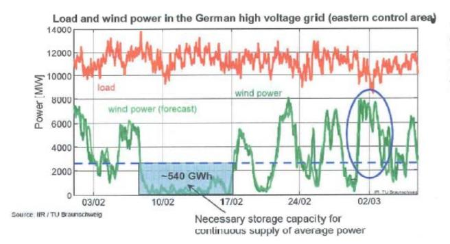
Significant power fluctuations from the mean and from forecasts
