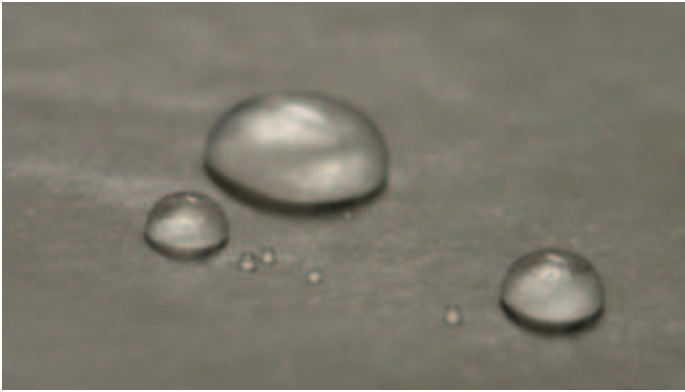
Water drops on waxed paper. Notice the nearly spherical shapes of the smallest drops.
