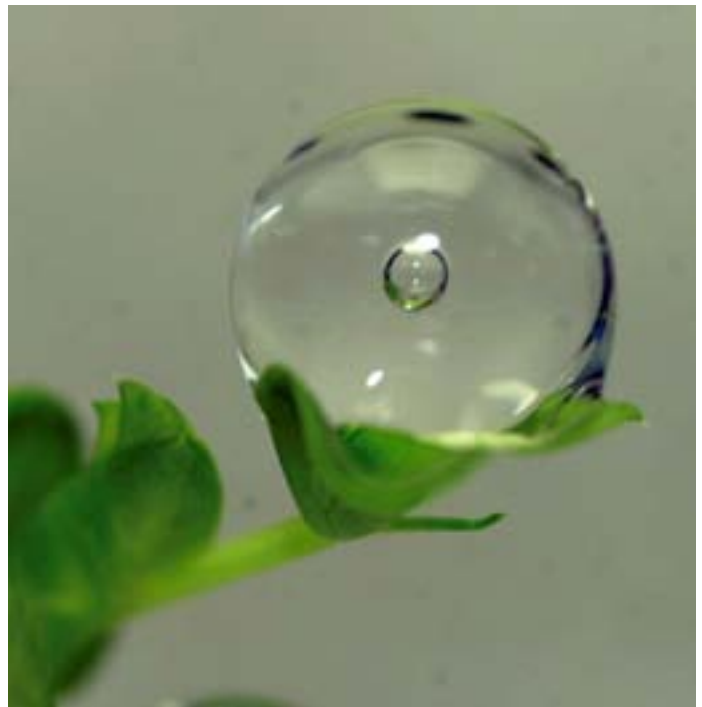
Large spherical water drop clinging to a leaf in a plant experiment on the International Space Station. Because buoyancy does not take place in microgravity, the bubble remains in the center of the drop.
