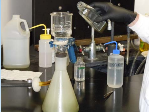
Pouring sample through filter
