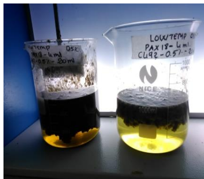
Figure 15: The difference in turbidity and colouring of the solution for a jar test evaluating the effect of temperature on COD removal. The sample at high temperature (60 – 70 °C) on the left vs the sample kept at room temperature (25 – 27 °C) on the right.
