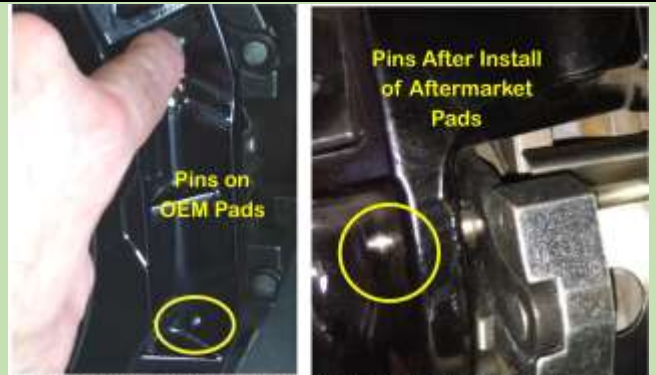
YouTube Video of PowerStop Pads showed an interesting Pin protrusion in the beginning of the video left and final install right. Note the difference. In addition in the video the installer used a hammer to make the pin flush but in that view the pins DID NOT PROTRUDE.
