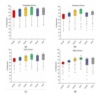
Figure 3: Variation in removal efficiency of (a) Phosphate (b) Ammonia (c) COD (d) BOD after the treatment with microalgal-bacterial consortia at 16 hours HRT
