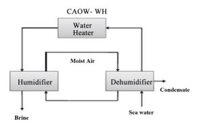
Figure 5. Close air-open water, water heated (CAOW-WH) system.
