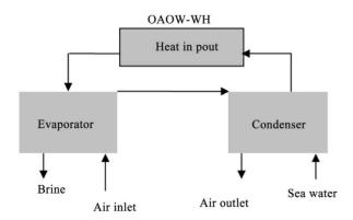
Figure 10. Open air open water air-heated (OAOW-WH) system.
