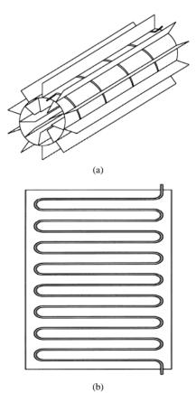
Figure 12. Sketch of the common type of condenser used in the desalination [6]. (a) Nawayseh (1996); (b) AI-Hallaj (1994).
