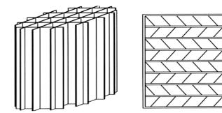
Figure 11. Shape of different wooden packing material used in the desalination by [6].
