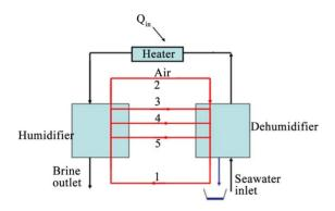
Figure 6. Multi-effect water-heated (CAOW) cycle.
