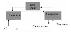
Figure 7. Open-air/closed-water cycle water heated (OACW-WH).
