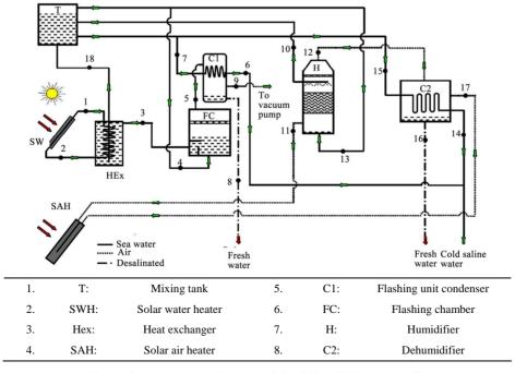
Figure 3. A schematic diagram of the (HDH/SSF) system [5].
