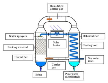
Figure 2. A simple humidification-dehumidification (HDH) process.
