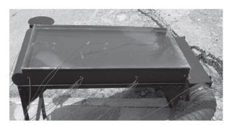
Figure 19. A view of the double-pass flat plate solar air heater [15].
