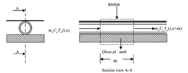
Figure 16. Thermal energy balance of differential section of solar water collector (one-temperature case).
