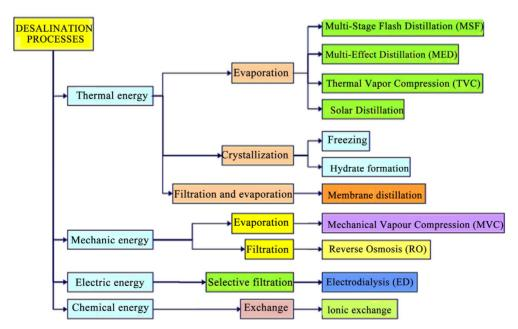
Figure 1. Different types of desalination processes.
