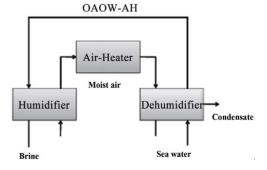
Figure 9. Open air open water air-heated (OAOW-AH) system.
