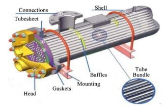
Figure 14. Shell and tube heat exchanger.
