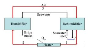
Figure 8. Closed air open water air-heated (OAOW-AH) system.
