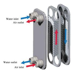
Figure 13. Plate fin tube heat exchange.
