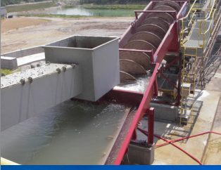
(Photo: Sand screw used to classify manufactured sand)
