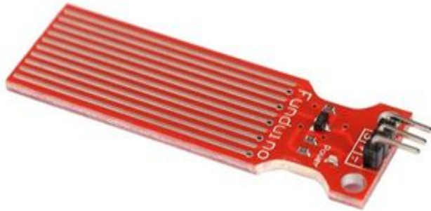
WATER LEVEL SENSOR
