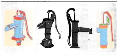
water is released to the upper side of plunger. On the next upward movement of plunger water is raised to pump head and discharged through the spout. By changing either the frequency of reciprocation or stroke length of the piston the discharge rate can be varied. The reciprocating pumps are available in various designs and models, which can be operated manually, with animal power and auxiliary power sources.
