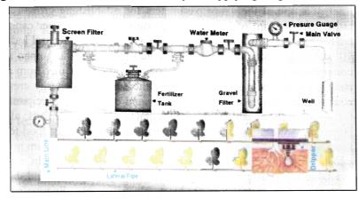
consumptive use of plants; therefore, the losses due to deep percolation, runoff and evaporation are minimized. Drip irrigation has been found suitable to orchard and vegetable
