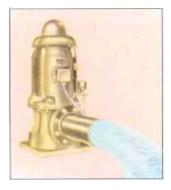
as stationary guide vanes guide upward the water thrown by the impeller to the periphery. The gradual enlarging vanes guide the water to the casing, thus converting kinetic energy into potential energy. Therefore, the turbine pump generates heads several times that of a volute pump. Turbine pumps are most effective for tube wells, and applications requiring high heads and discharge. A well-maintained pump provides trouble free service for several years.
