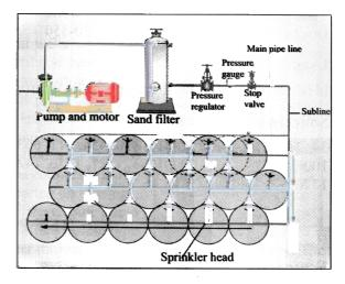
Sprinkler system is broadly classified as rotating head system and perforated pipe system. The rotating head system may be portable, semi permanent, solid set and permanent system. Usually portable system is more popular which can be moved after applying one irrigation to the crop to another area and also requires less initial investment. The perforated
