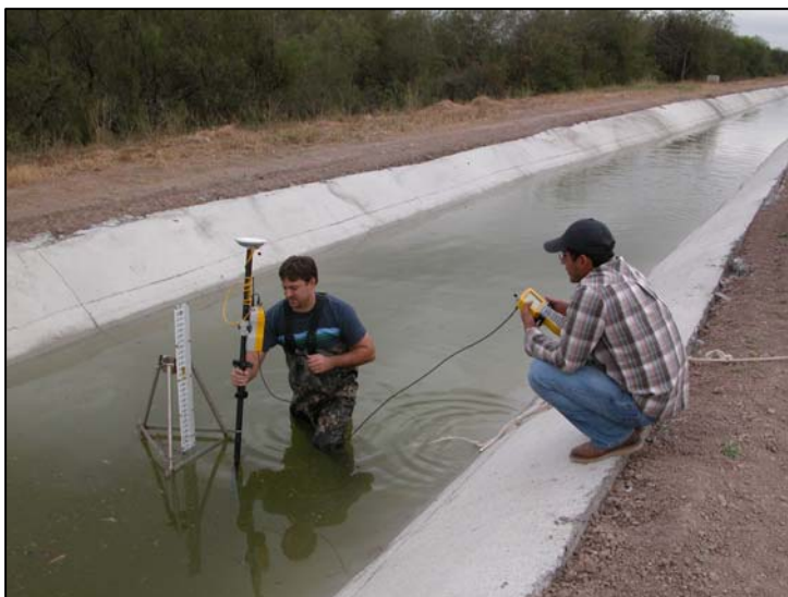
Figure 4. Survey-grade GPS equipment used to determine the cross-section of the canal (Lateral A).
