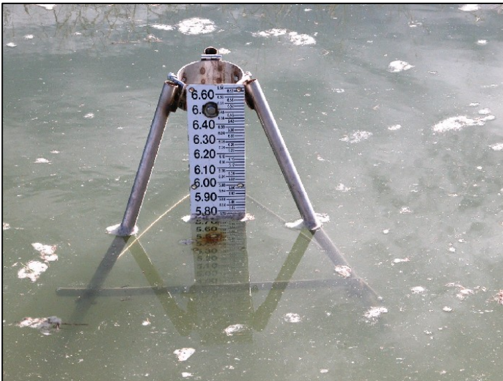
Figure 3. Staff gage stands are place in the center of the test segment.
