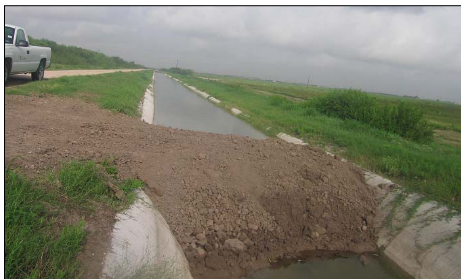
Figure 6. Earthen dam on Lat. A-7. (Test SJ15)
