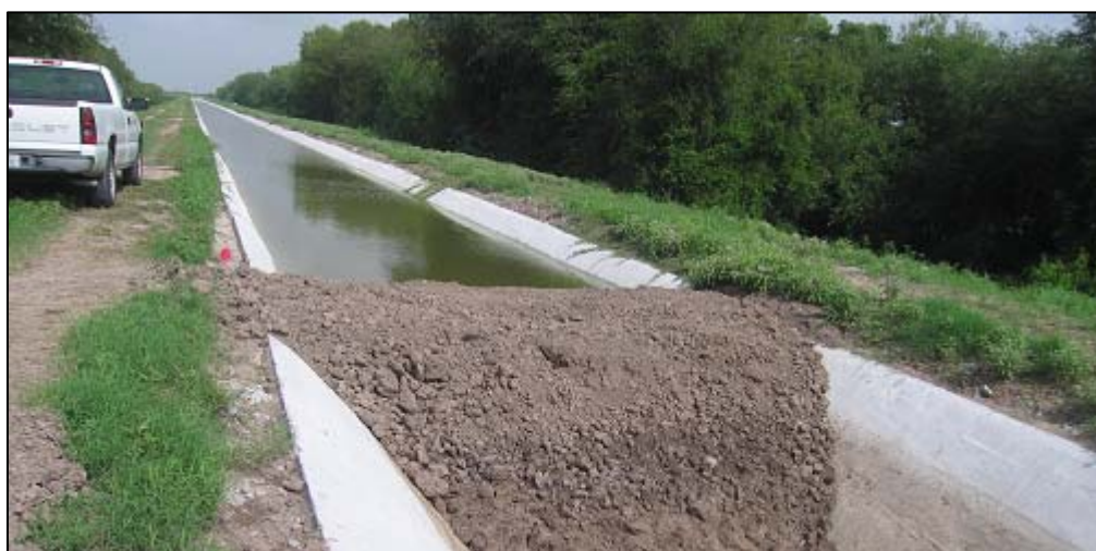
Figure 10. Earthen dam on Lat.A-8. (Test SJ12)
