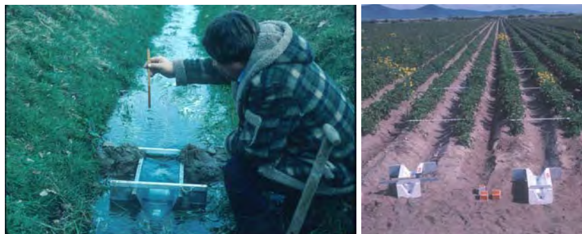
Figure 7. — Portable RBC Flumes Measure Flow in Drains and Furrows.
