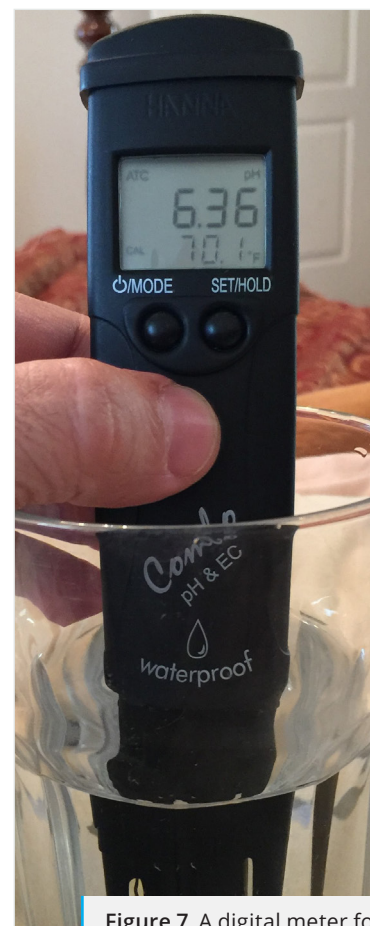
Figure 7. A digital meter for measuring pH, electrical conductivity (EC), and the temperature of water.
