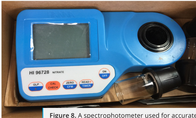
Figure 8. A spectrophotometer used for accurate measurements of various nutrients in water. This one is used for measuring nitrate.
