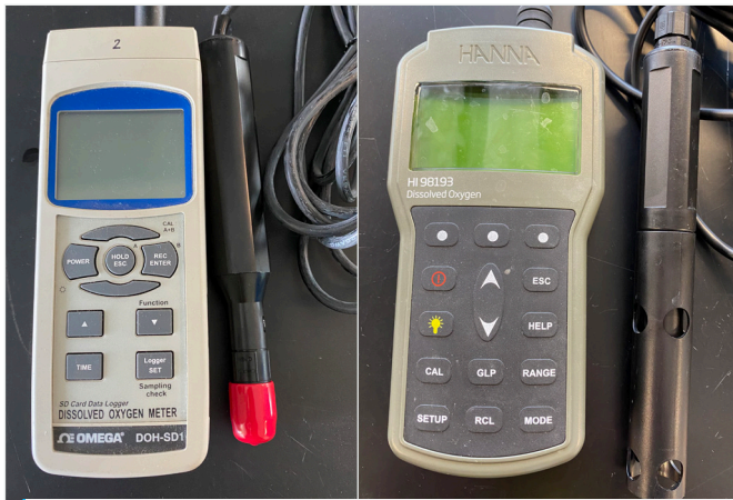
Figure 1. Two examples of meters available on the market for accurate measurements of dissolved oxygen in the water.
