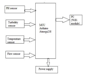
Fig: Block diagram of our project
