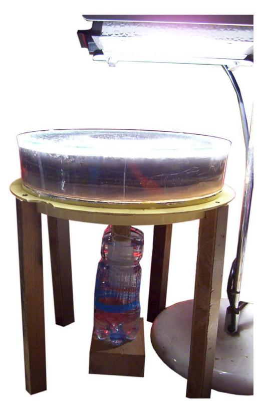
Situation: the output pipe of the model is inserted in a bottle full of water
