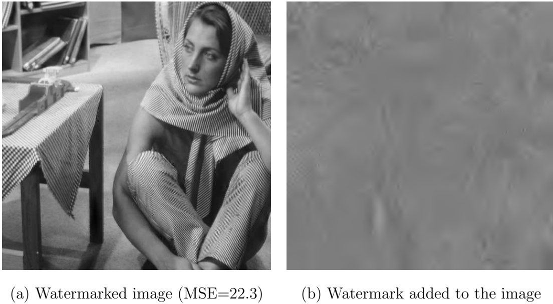
Fig. 1.7. A watermarked image (a) and its watermark (b) for a DWT spread spectrum watermarking.
