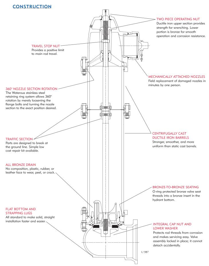
Fully complies with AWWA C502 and is available in configurations which are UL Listed and FM Approved.
