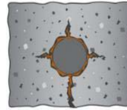
FURTHER CORROSION. SURFACE CRACKS. STAINS.
