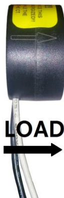
Fig. 2: Current transformer (CT) orientation
