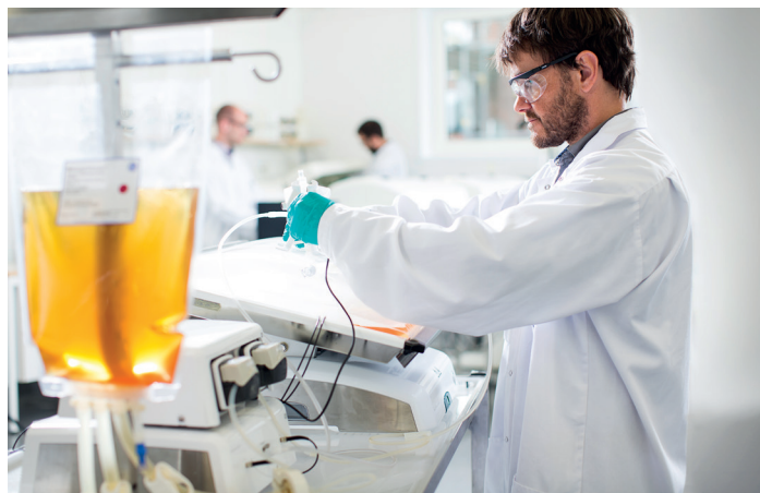
Fig 3. Cellbag equipped with ReadyMate connectors facilitates quick aseptic connection to downstream operations.
