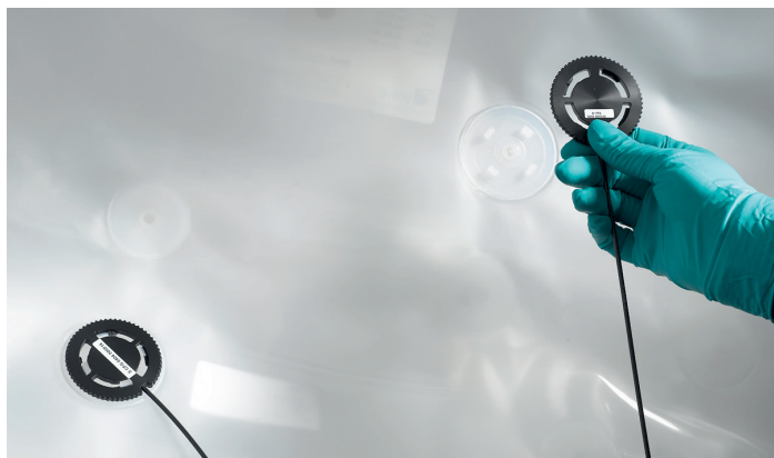
Fig 4. The optical sensor is embedded in the underside of the Cellbag bioreactor. Shown here is the bag adapter/optical fiber cable attached to the bag port.
