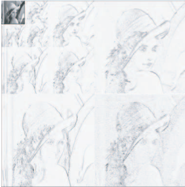
FIGURE 4. Wavelet Decomposition of an Image Component - 3rd Level Decomposition. The image has been modified: the average detail has been lightened and the horizontal, vertical and diagonal details are shown as negative images with a reversal of white and black, because of constraints of the printing process.
