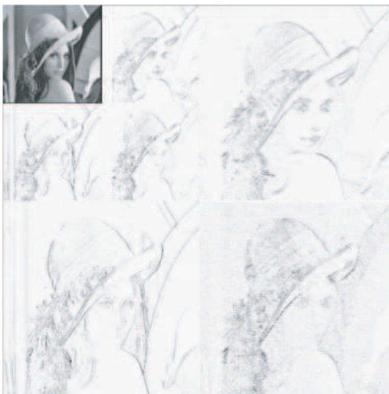
FIGURE 3. Wavelet Decomposition of an Image Component - 2nd Level Decomposition. The image has been modified: the average detail has been lightened and the horizontal, vertical and diagonal details are shown as negative images with a reversal of white and black, because of constraints of the printing process.
