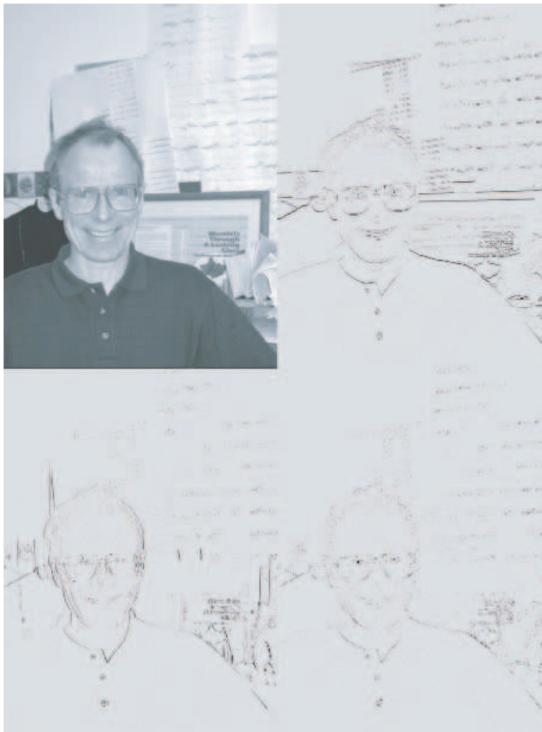
FIGURE 6. Wavelet Decomposition of an Image Component - 1st Level Decomposition. The image has been modified: the average detail has been lightened and the horizontal, vertical and diagonal details are shown as negative images with a reversal of white and black, because of constraints of the printing process.
