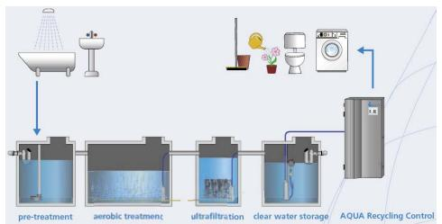
Figure D-2: A typical domestic greywater recycling system
