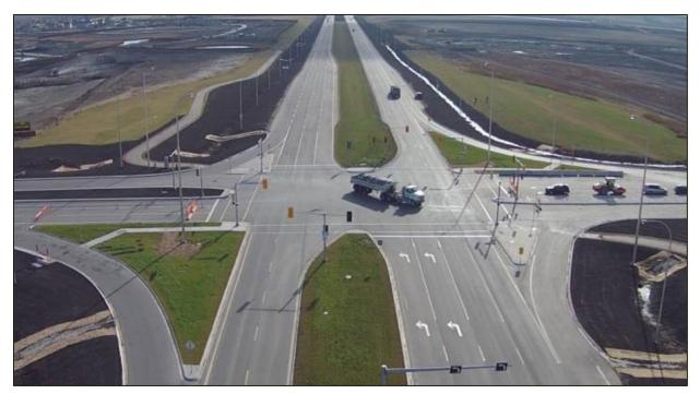
Figure 4: Smart Channels going from Major to Minor Roadway.
