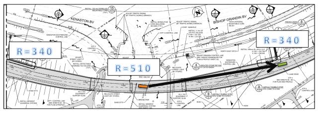
Figure 8: Adequate stopping sight distance achieved through combination of geometric changes.
