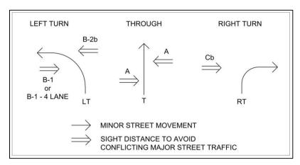
Figure 2: Sight Distance Parameters for Turning Movements from Stop Condition.
