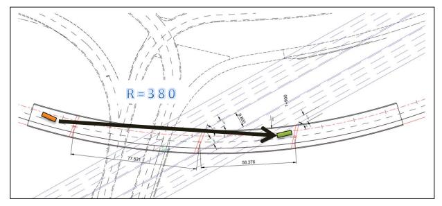
Figure 7: Inadequate stopping sight distance due to visual interference from F-shape barriers.
