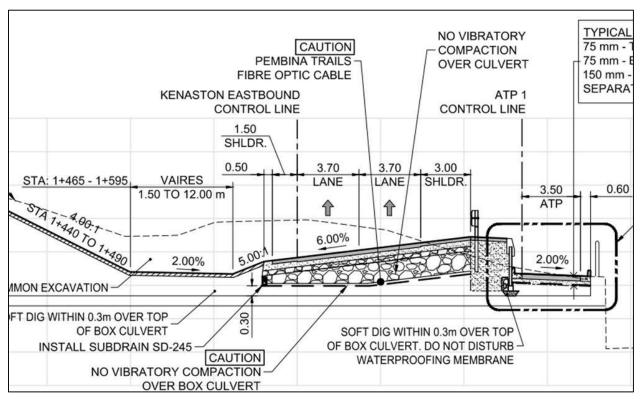
Figure 12: Cross-section illustrates MSE wall required to drop grade to fit AT path on box culvert structure. Guardrail required for protection from drop off.
