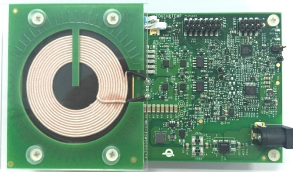
Figure 1. WCT-15W1COILTX reference board
