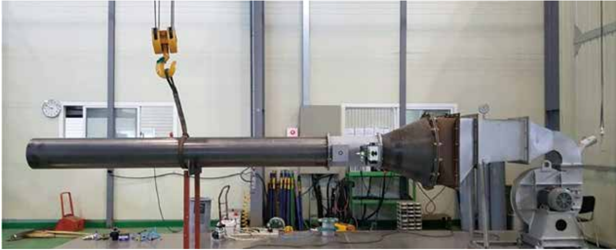
Damper leakage quantity test
