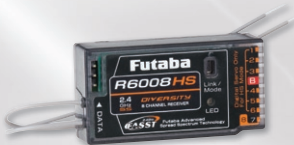
R6008HS 8-Channel High-Speed Dimensions: 1-3/4 x 7/8 x 1/2 in (47 x 25 x 14 mm) Weight: 0.48 oz (13.54 g); Weight w/o case: 0.33 oz (9.32 g) FUTL7639
