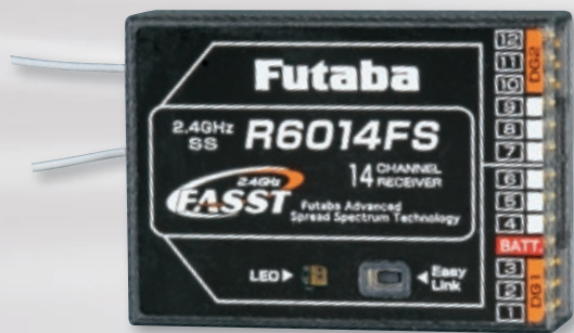
R6014FS 14-Channel Dimensions: 2-1/16 x 1-1/2 x 5/8 in (52 x 38 x 16 mm) Weight: 0.72 oz (20.8 g) FUTL7644
