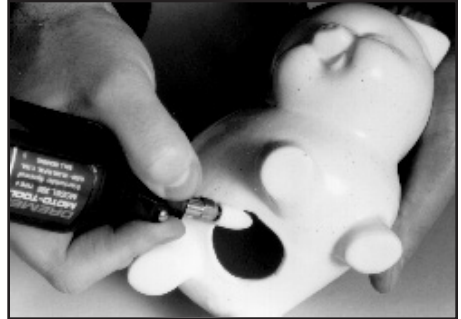
Flame #9022 is excellent for making existing holes in ceramic bisque slightly larger.
