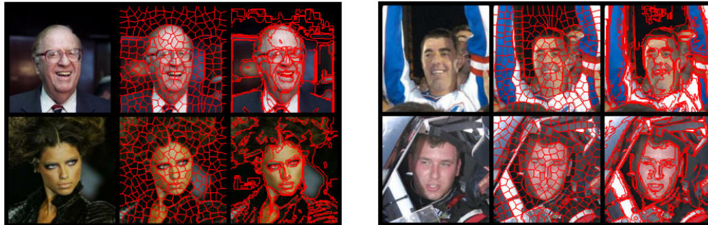
Figure 2.3: Examples of superpixels. The left column is the original image, the middle column is the Mori segmentation ( N_{sp}=100 , N_{sp2}=200 , N_{ev}=40 ), and the right column is the Felzenszwalb-Huttenlocher segmentation ( \sigma=0.5 , K=100 , \min=20 ).
