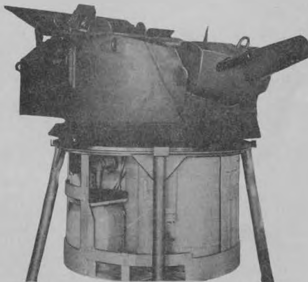
TURRET BASKET ASSEMBLY FOR MODEL Q FLAME THROWER
