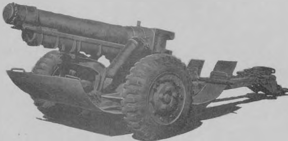
105MM. HOWITZER CARRIAGE, M3A1 (AIRBORNE), MODIFIED BY USE OF SKID PANS
