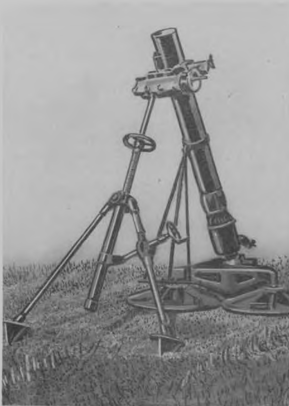
155MM. MORTAR, T16 (RIFLED BORE), AND MOUNT, T9, WITH LONG BASE PLATE, IN FIRING POSITION
