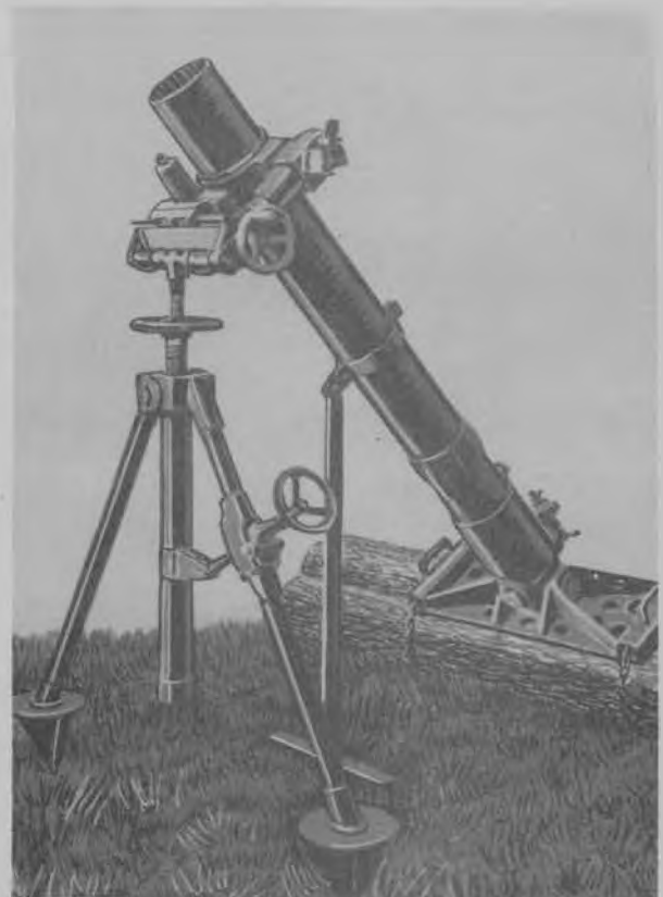
155MM. MORTAR, T17 (SMOOTH BORE), AND MOUNT, T10 ON BASE PLATE FOR SOFT GROUND, IN FIRING POSITION
