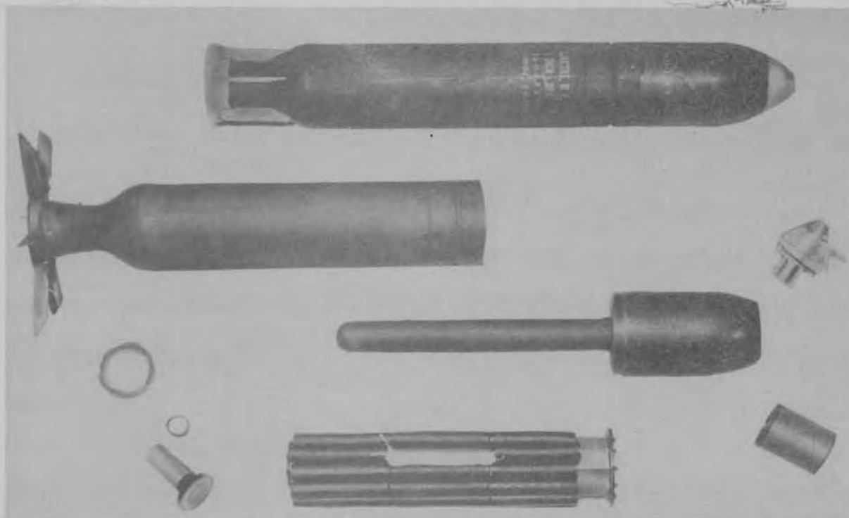
ROCKET, 4.5", M8, WITH FUZE, ROCKET, P.D., M4, DISMANTLED TO SHOW MOTOR BODY, TAIL LOCKING SHELL, AUXILIARY BOOSTER, FUZE PRIMER CUP AND PROPELLANT CHARGE IN CUP
