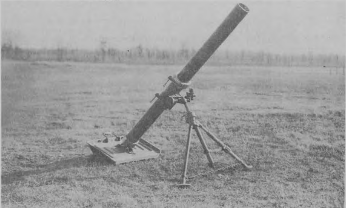
105MM. MORTAR, T13E6, AND MOUNT, T12, IN FIRING POSITION
