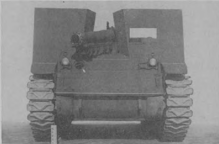
105MM. HOWITZER, M3A1, ON LIGHT TANK CHASSIS, M5. GUN AT MAXIMUM DEPRESSION
