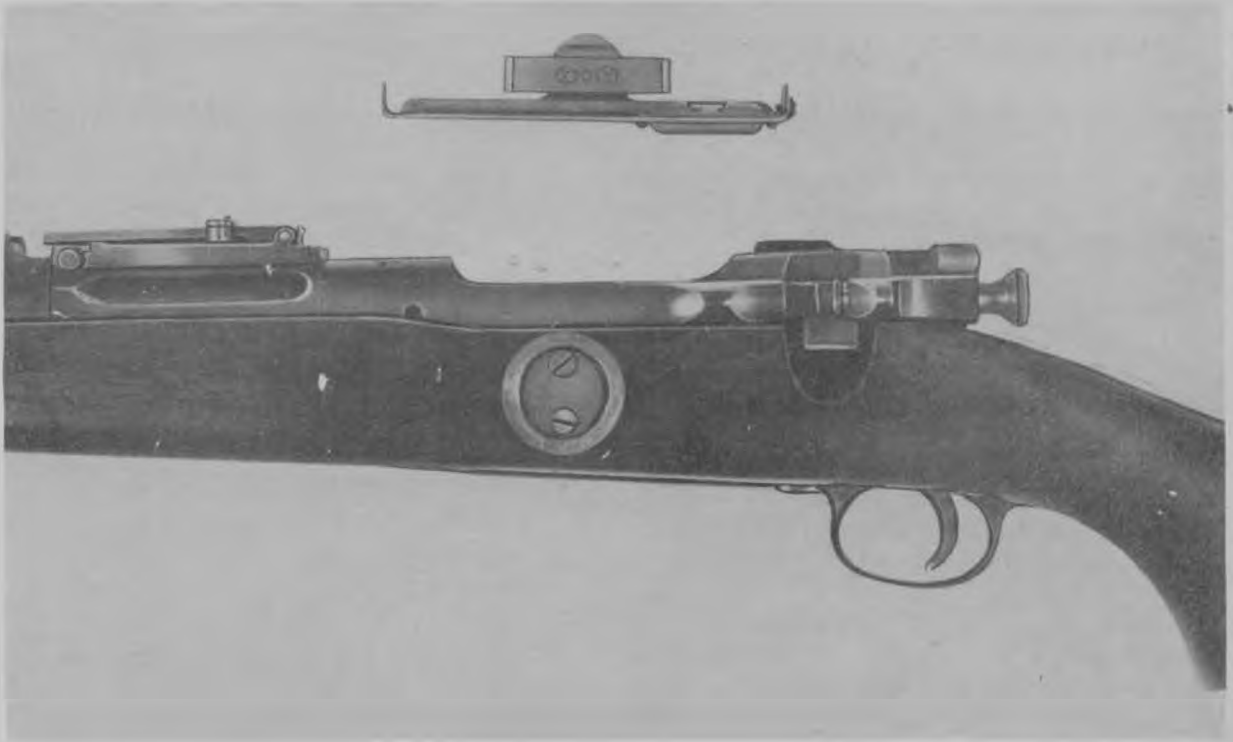
SIGHT, GRENADE LAUNCHER, T59, SIGHT REMOVED FROM RIFLE, MOUNTING PLATE REMAINS ATTACHED TO STOCK
