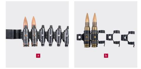
Note: (a) Non-disintegrating belt (7.62  $\times$  39 mm cartridges in a belt used by the Soviet RPD LMG); (b) Disintegrating belt and links (7.62  $\times$  51 mm cartridges in M13 links, as used by the American M240 general-purpose machine gun, for example). Source: Jack Dutschke/ARES
