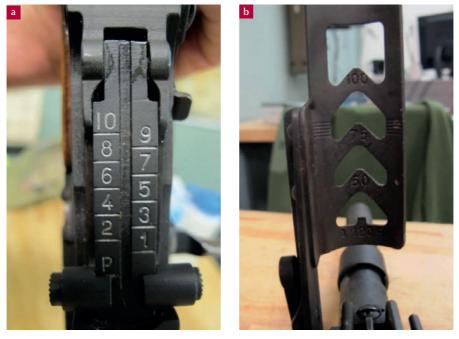
Note: (a) Rear sight markings on the adjustable rear sight of a Romanian Pistol Mitralieră md. 1963 self-loading rifle. A 'P' appears in place of zero, in bottom left position. (b) Markings on a folding rifle grenade leaf sight on a French MAS Modèle 1936-51 bolt-action rifle.
