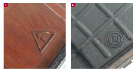
Note: (a) IZHMASH and (b) Arsenal JSCo markings on Russian and Bulgarian AK-pattern 7.62  $\times$  39 mm magazines, respectively.
