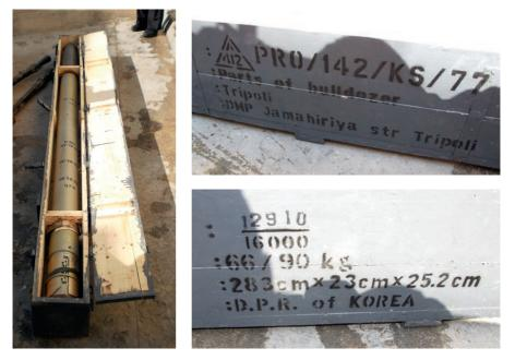
Note: Markings in the top right-hand image indicate that the crate contained 'Parts of bulldozer', when it in fact contained a 122 mm high-explosive fragmentation (HE-FRAG) artillery rocket. Small arms are also sometimes packaged in a similar fashion.
