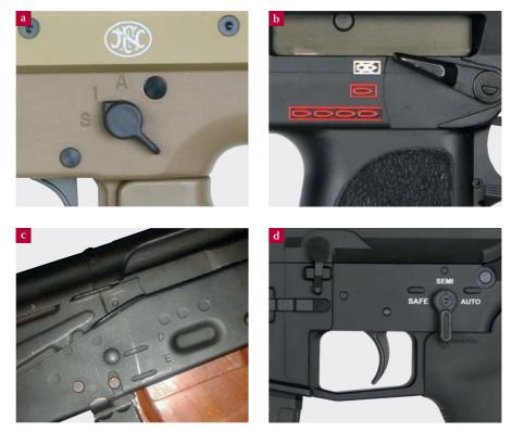
Note: (a) Markings (S, 1, A) on a Belgian FN Herstal SCAR-L self-loading rifle. (b) Pictographic markings on a German Heckler & Koch MP7 SMG. (c) Markings (D, E) on an East German MPi-KM self-loading rifle. (d) Markings (SAFE, SEMI, AUTO) on a British LANTAC LA-M4 self-loading rifle. Sources: ARES (n.d.); N.R. Jenzen-Jones/ARES
