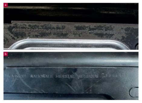
Note: (a) Factory marking reflecting manufacture prior to November–December 1971, marked: 'FABRIQUE NATIONALE D'ARMES DE GUERRE–HERSTAL–BELGIQUE'. (b) Factory marking reflecting manufacture after November–December 1971, marked: 'FABRIQUE NATIONALE HERSTAL BELGIQUE'. Source: Jenzen-Jones and Spleeters (2015)
