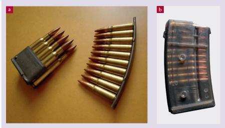
Note: (a) Examples of en bloc (left) and charger/stripper clips (right). (b) A (transparent polymer) removable box magazine for comparison. Source: Wikimedia Commons/Amenhtp/Rama
