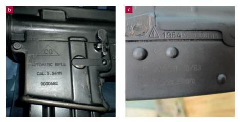
Note: (a) Markings ('Tabuk' and 'Cal. 7.62×39mm') on the right side of the rear sight block of an Iraqi Tabuk self-loading rifle. (b) Markings ('CQ' and 'CAL. 5.56MM') on a Chinese CQ self-loading rifle. (c) Markings ('WASR 10/63' and 'Cal. 7.62x39mm') on a Romanian GP WASR 10/63 semi-automatic rifle, rebuilt to Pistol Mitralieră md. 1963 standard. These are post-production markings engraved by an importer.
