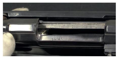
Note: The marking reads simply '7 M M'. After a chamber cast and test-fitting of a dummy cartridge, it was determined to be chambered for 7 mm Mauser (7  $\times$  57 mm). Source: Ferguson (2017a)
