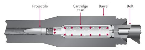
Note: The cartridge case and bolt face provide a gas seal. Adapted from: Chinn (1955, p. 4)
