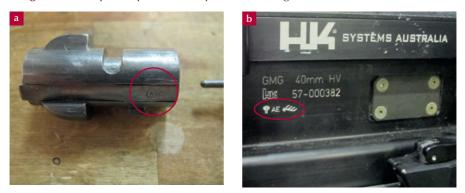
Note: (a) Proof marks on the bolt head of a Russian Mosin-Nagant Model 1891/30 bolt-action rifle. (b) Proof and inspection marks on a German Heckler & Koch grenade machine gun. Source: N.R. Jenzen-Jones/ARES
