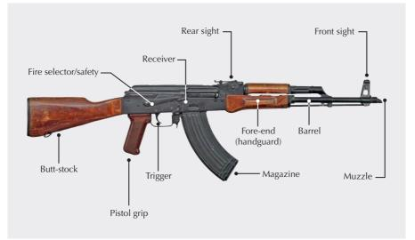
Note: With handguns, what might be termed the 'receiver' is typically referred to as a 'frame'. The slide of a self-loading pistol is similar to the 'upper' receiver of a rifle. Pistols by definition lack a butt-stock (ARES, 2017). Source: Chloe Tousignant/ARES
