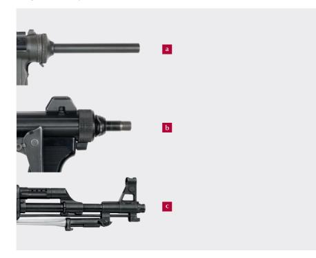
Note: (a) A bare muzzle on a US Guide Lamp M3 SMG; (b) A threaded muzzle on an Italian Beretta Model 12S SMG; (c) A thread protector or 'muzzle nut' on a Chinese Type 56-1 self-loading rifle (note also the under-folding integral bayonet).
