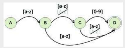
Output:[a-z][[a-z]|[a-z][[a-z]|[0-9]]] (can be simplified, and also the FSA)
